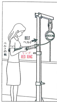
FASTEN THE BELT WITH RED RING IN YOUR FRONT POSITION. AND TIGHT THE BELT.
